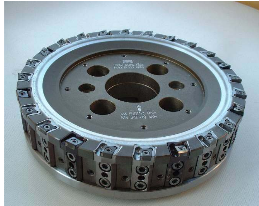
Mill with PCD cutting edges
