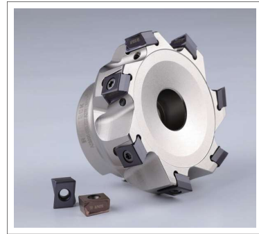
ASM90-LN13, shoulder milling cutter with tangential mounted inserts with 4 cutting edges, applied for machining component features on turbine casing.
