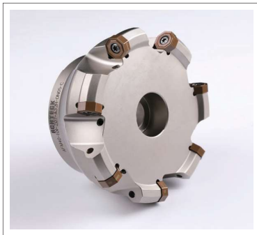
AFM40-ON05-C-45, with 45° approach angle, wiper inserts with 16 cutting edges, For finishing of the flange face of turbine casing.
